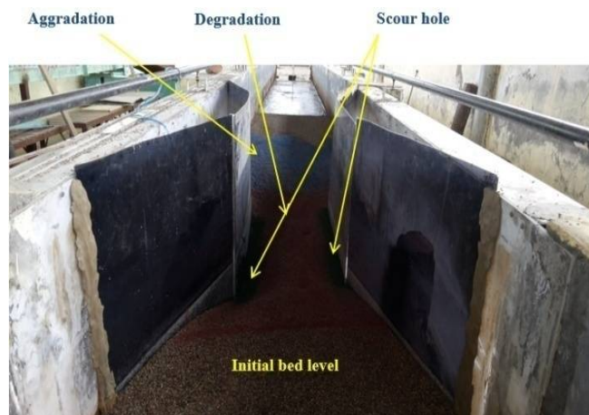
Fig. 4: Shows the plan of bed profile (CR = 0.3, \theta = 75^\circ )
